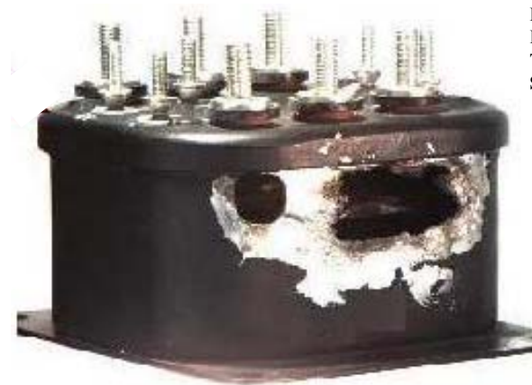
Damage from whiskers induced metal vapor arc in relay
