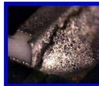
Cracked solder joint open circuit
