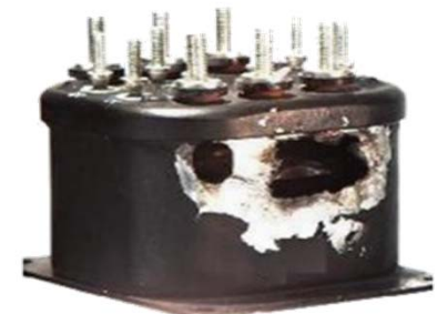
Electromagnetic relay short circuit; 115V metal vapor arc in air
