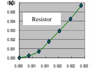
Solder strain as a fn of PWB curvature
