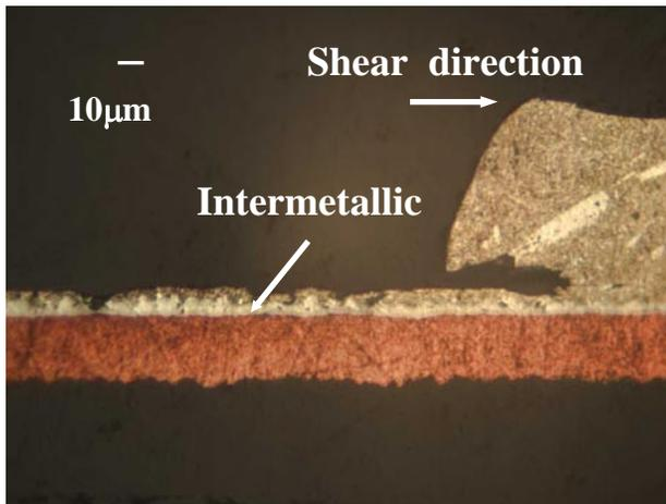
Shear testing failure at the interface between SnAgCu and intermetallic on HASL<sup>T</sup> after aging 100 hours at  $0.9T_m$  (168°C)
