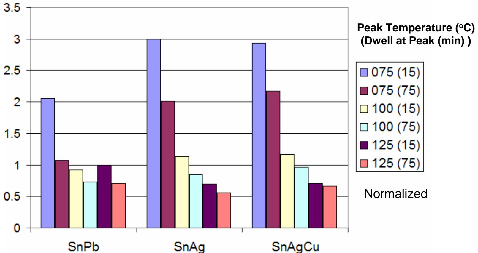
For the Pb-free solders, increasing the average cyclic temperature showed a decrease in time to failure. As can be seen in the above chart, the behavior of the SnPb solder at the 100 and 125°C peak temperature shows non-monotonically decreasing behavior.
