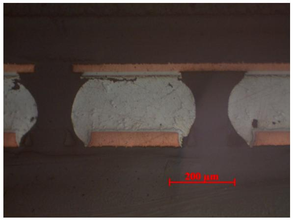
Section of a 192 IO CABGA with SAC305 solder sphere attached with SAC305 solder. Removed after 4257 cycles under -15 to 125°C, 60 minute dwells.
