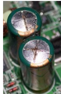
Change of electrolyte in electrolytic capacitors produced excessive bulging and early failure
