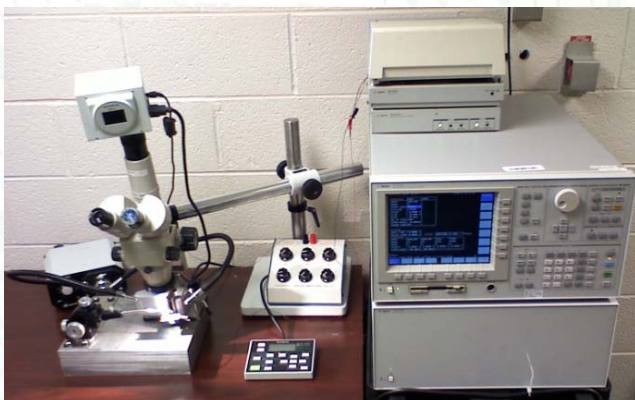
Figure 1. Experimental setup for measuring the breakdown voltage
