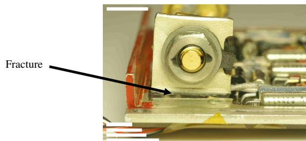
**Fig. 3: Failed Aluminum Bracket.**
